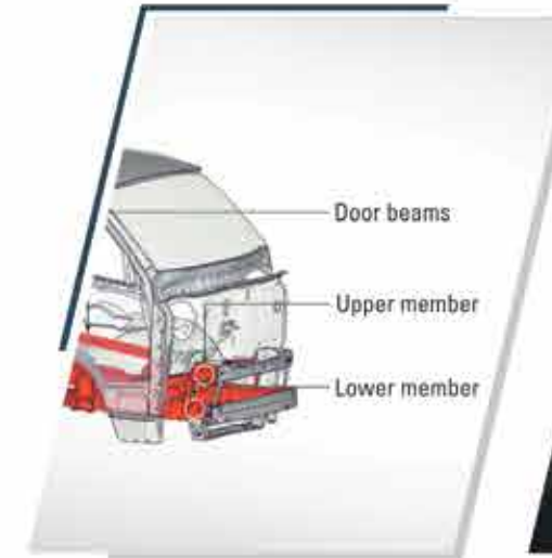
New upper and lower front frame members
